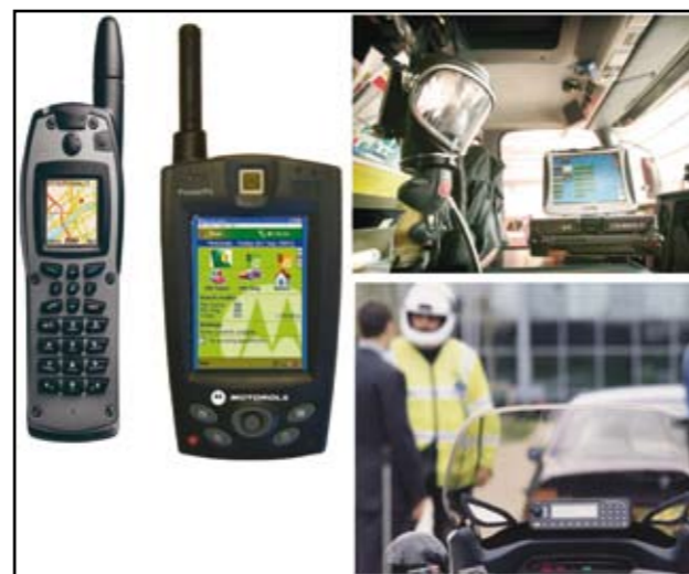
Fig. 4: Handheld and vehicle-mounted TETRA mobile stations
